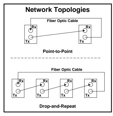
Note that in single Master/multiple Slave installations, for proper operation, the DX-7101 specifically connected to the Master must be set to the Point-to-Point mode, while the slaves are set for drop and repeat.
