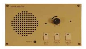
The INCX-4001 consists of an audio transceiver designed to implement a complete fiber optic intercom system. The unit can be used in point-to-point applications, or as a simple party line intercom. Both push-to-talk and hands-free operation are supported and a jack is provided for use with an external headset. The unit may be used on a desk top or mounted to a wall as required.
