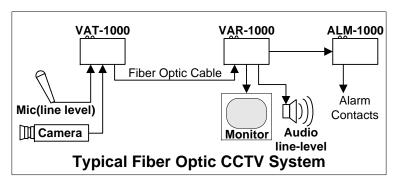
Note that when there is a loss of signal carrier, usually due to broken fiber or excessive optical path loss, the Alarm indicator will light and the Link indicator will go off. The alarm switch cannot disable the function of the indicator lights.
