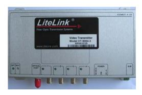
The VT/VR-9004 system consists of the VT-9004 transmitter and VR-9004 receiver and will transmit four separate channels of high quality base-band video on one fiber in accordance with NTSC, PAL and SECAM specifications.
